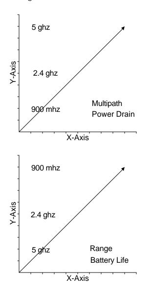
increases as the frequency increases. "Multipath Fading" can be simply understood as the radio waves canceling themselves out due to interference
