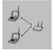
Infrastructure or BSS (Basic Service Set) This is a configuration where you have any number of wireless clients and a single access point The access point is the intermediary between the devices
