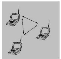
Peer to Peer, Ad-Hoc, IBSS (Independent Basic Service Set), All of these terms mean the same thing. Basically device to device mode. There is no central point in this configuration.
